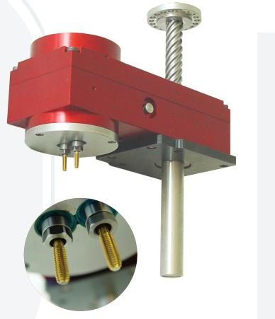
These models are commonly used to tap electrical components such as contactors, etc... they are the best solution for applications with small distance centers and small tap sizes within a high-speed press.
