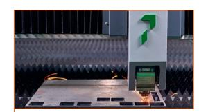
Full auto focus cutting head with easy access for cleaning/changing of quartz window. Focus position from program control assists in optimum piercing and cutting conditions.
